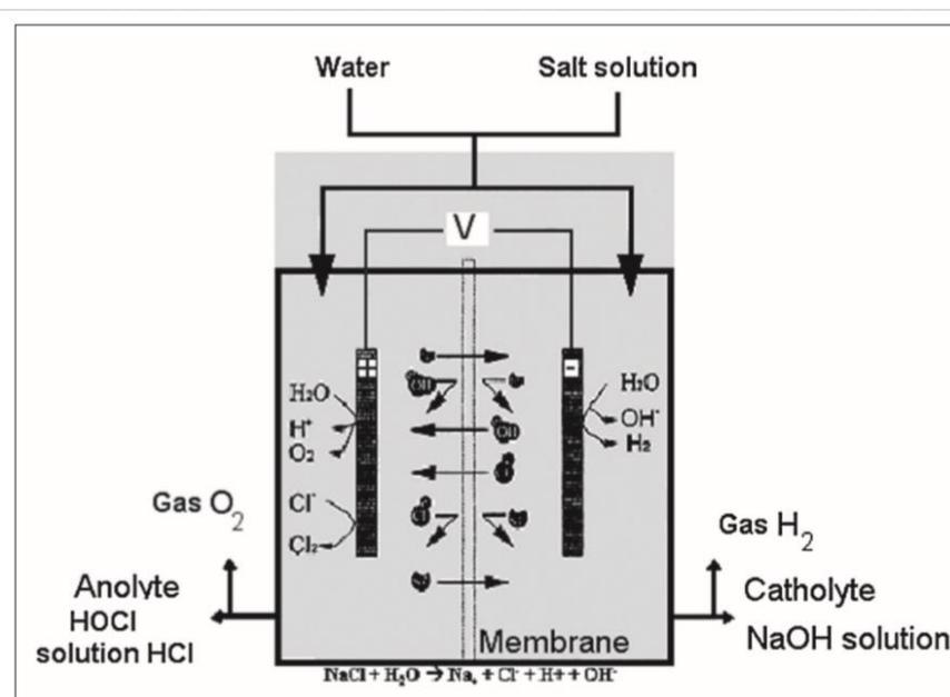
**Figure 1: Device for electro-chemical activation of water<sup>2</sup>**
